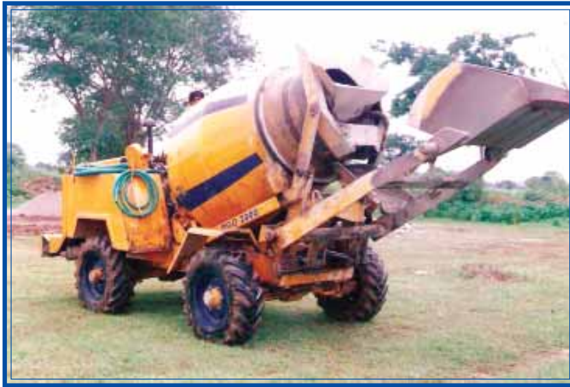
FIG: 21 SELF-LOADING MOBILE CONCRETE MIXER
