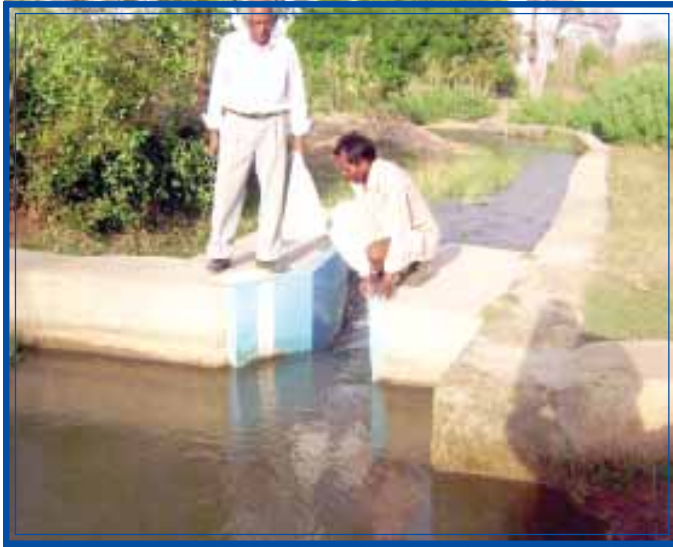
FIG:23 MEASURING DEVICE Measuring discharge through a calibrated scale
