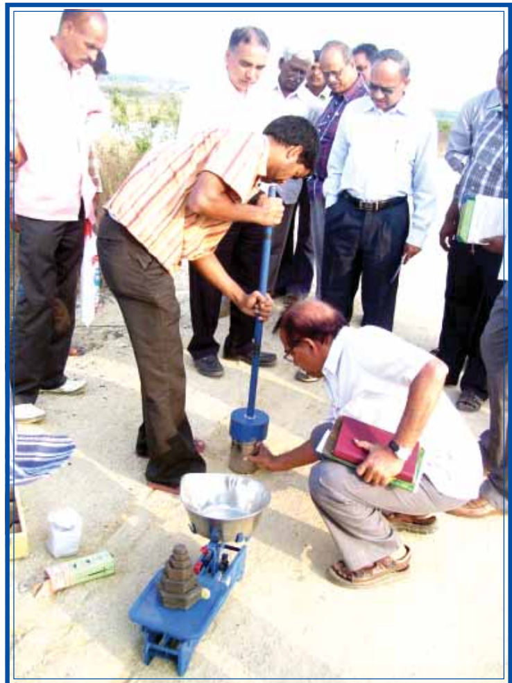
FIG: 6 PROCTOR'S DENSITY TEST BEING CONDUCTED ON CONSOLIDATED BUND
