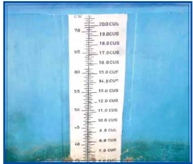
FIG:24 CALIBRATED SCALE ON CUT-THROAT FLUME
